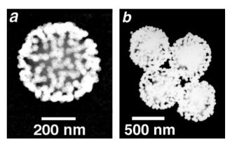
Fig. 1 TEM images (Philips EM-400, 100 kV) of  $Au/SiO_2$  superparticle ensembles. Diameters (in nm): (a) 30/430; (b) 60/550.
